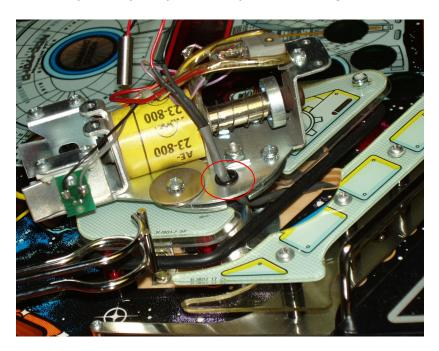
10. Take new cannon cover, turn upside down and **CAREFULLY** insert front of laser (first) into cannon cover molded hole, **NOTE**, keep laser's wires parallel to wire slot, (see below picture) and very carefully push in the laser, then push down until fully seated.
