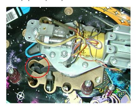
6. Push up from the bottom of playfield the laser with attached gray cable, (about 6 inches) and then up through the empty hole in the metal cannon base, shown below. DO NOT PULL ON THE LASER WIRE LEADS, AS THEY COULD PULL OUT!
