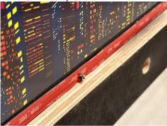
4. The Saucer and Martian wiring assembly is below the baseboard. Thread the wiring assembly through the hole in the backboard.
